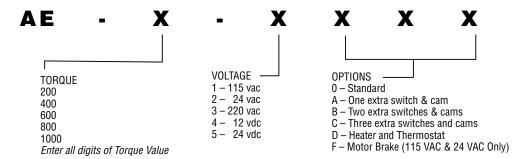
Note: AE will always be the first two characters of the part number, all digits from torque value must be entered into part number (i.e. 400, 1000 etc.) Only use one digit for voltage depiction (i.e. 1-5). For the options listing you may use more than one character, up to three, (i.e. O, AD or BD etc.)
